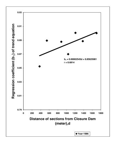
Fig. 3. Relation between regression coefficients of accretion height equations and the closure distance
