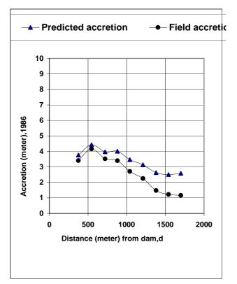
Fig. 5. Predicted and field accretion with respect to distance, 1986
