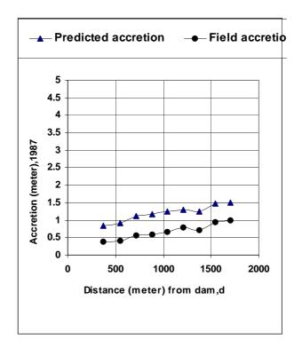
Fig. 6. Predicted and field accretion with to respect to distance, 1987
