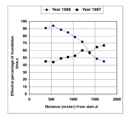
Fig. 4. Impact of dam (in terms of effective percentage of inundation time for deposition of sediment) with respect to its distance
