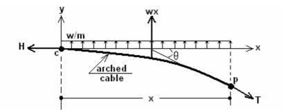
Fig.4 The forces acting on a portion of an arched cable.
