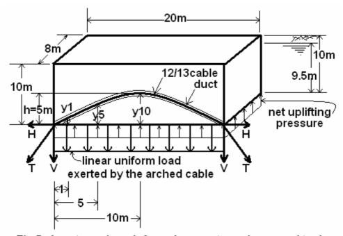
Fig.5- A rectangular reinforced concrete underground tank, stabilized against floatation by two arched cables.
