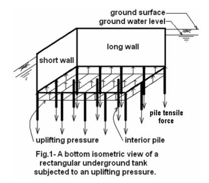
For a typical interior pile supporting an underground reinforced concrete tank with the following properties, 10m depth, 0.5m thick walls, and 2m on centre of piles, it is easy to calculate that: this interior pile will support a compression of 460kN, when the tank is filled with water and the ground water level falls below its floor, while it must be prepared to resist a pulling up tensile force of 300kN, when the tank is empty and the ground water level rises to its maximum.
