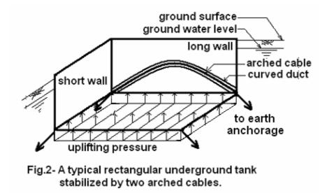
Uplifting pressure due to the displaced underground water is a uniformly distributed upward pressure applied to the tank floor. If the two long walls of the tank can be fixed in their positions, and this is the aim of this research, then the design of the tank floor will be similar to a one way slab subjected to an upward uniform load.
