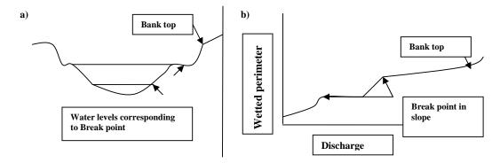
Figure 1.1. Wetted-perimeter method: (a) hypothetical channel cross-section and (b) graph of wetted perimeter versus discharge. Breakpoints in slope indicate the maximum available fish habitat for the least amount of water, until the next breakpoint (Davis and Hirji, 2003).
