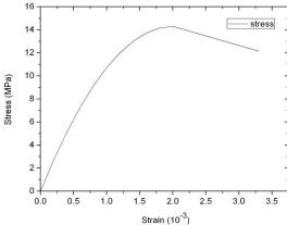
Figure 3. MISO curve of the concrete
