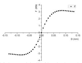
Figure 1. The load-displacement relationship of the spring element along the longitudinal direction
