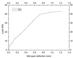
Figure 9. Load-displacement curve with the spring element
