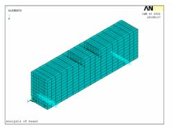
Figure 7. Consolidated supported beam model
