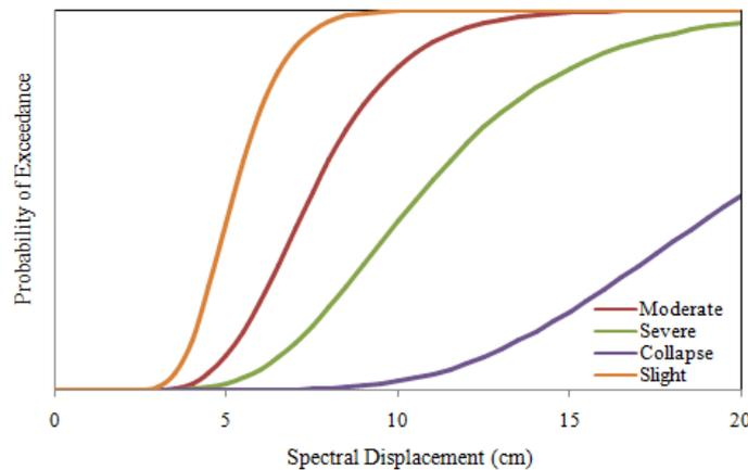
Fig. 12. Fragility Curves of Bare Frame Model
