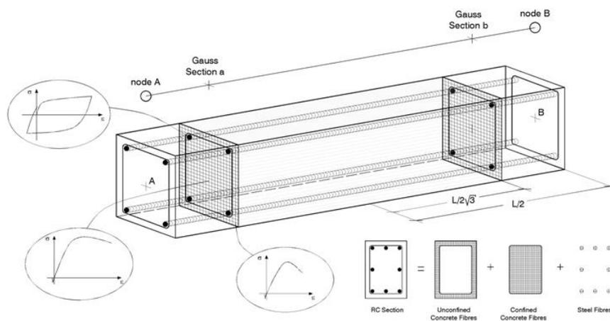
Fig. 3. Reinforced Concrete Section (Source: SeismoSoft v7.0, 2015)
