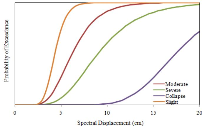
Fig. 13. Fragility Curves of RC Frame with Infill walls model.
