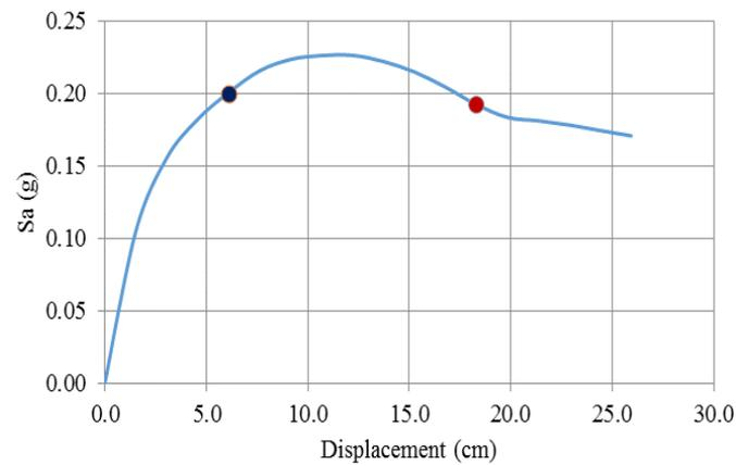
Fig. 11. Capacity curve for Infill model.
