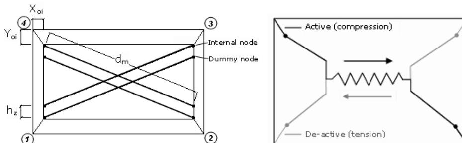
Fig. 2. Infill panel element: compression struts and shear strut (Crisafulli, 1997)
