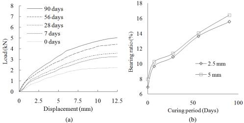
Fig. 5. (a) Load-displacement curves for the reference mix with cuing period, (b) Variation of bearing ratio for the reference mix with curing period.
