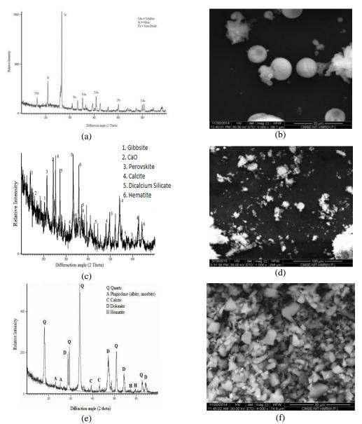
Fig. 1. (a) X.R.D of flyash, (b) SEM of fly ash (30kV, X5000, 20 $\mu$ m), (c) X.R.D of redmud (d) SEM of redmud (30KV, X1000, 100 $\mu$ m), (e) X.R.D of marble dust, (f) SEM of marble dust(30kV, X4000, 74.6 $\mu$ ).
