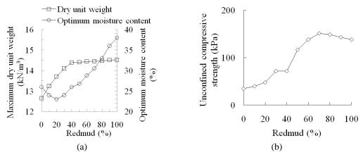
Fig. 2. (a) Variation of moisture content and maximum dry unit weight with varying percentage of redmud (b) Variation of unconfined compressive strength with percentage of redmud.
