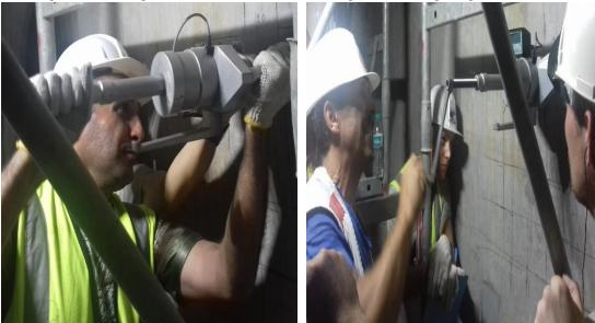
Fig. 7(a). Set-up of pull-out test instrument.
