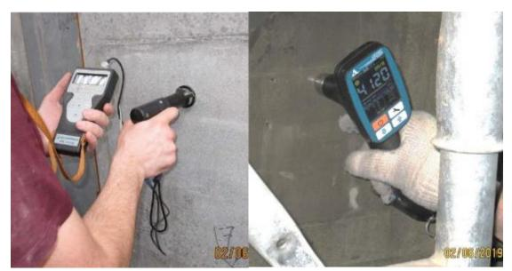
Fig. 3. Shock pulse test on annular floor walls. Fig. 4. Ultrasonic measurement of concrete of
