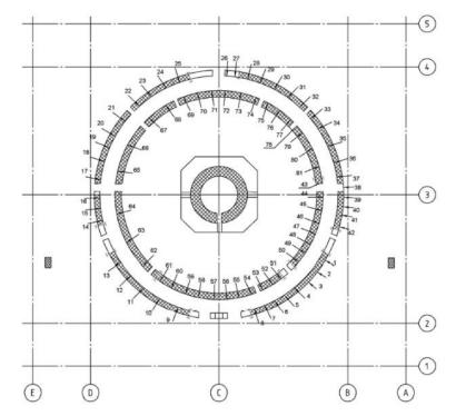
Fig. 1. Different sections of inner and outer corridor wall have been numbered for NDT.
