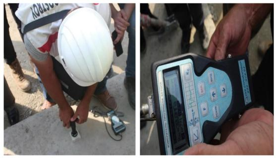
Fig. 2(a). Checking the shock impulse machine using reference prism.
