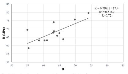
Fig. 10. Calibration dependence graph between shock pulse test & pull-out test results.
