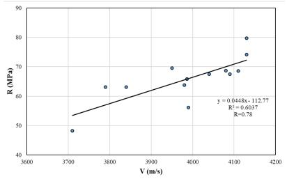
Fig. 11. Calibration dependence graph between ultrasonic test & pull-out test results.
