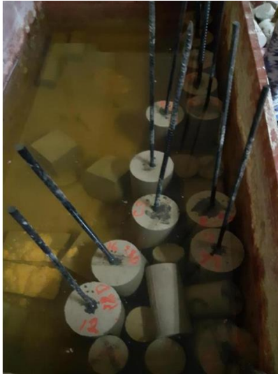
Fig. 2. Curing by ponding.
