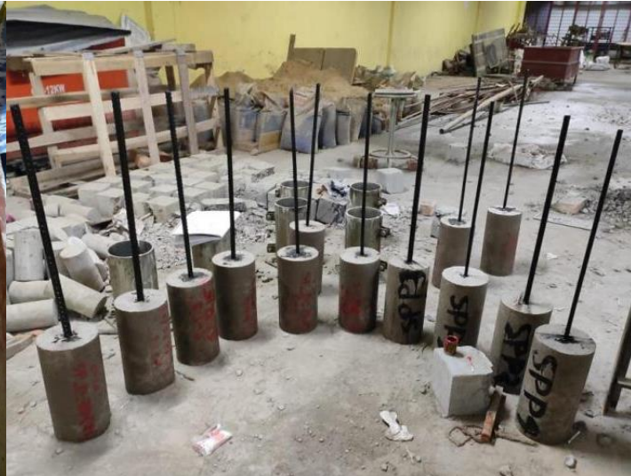
Fig. 3. Pullout specimens preparation.
