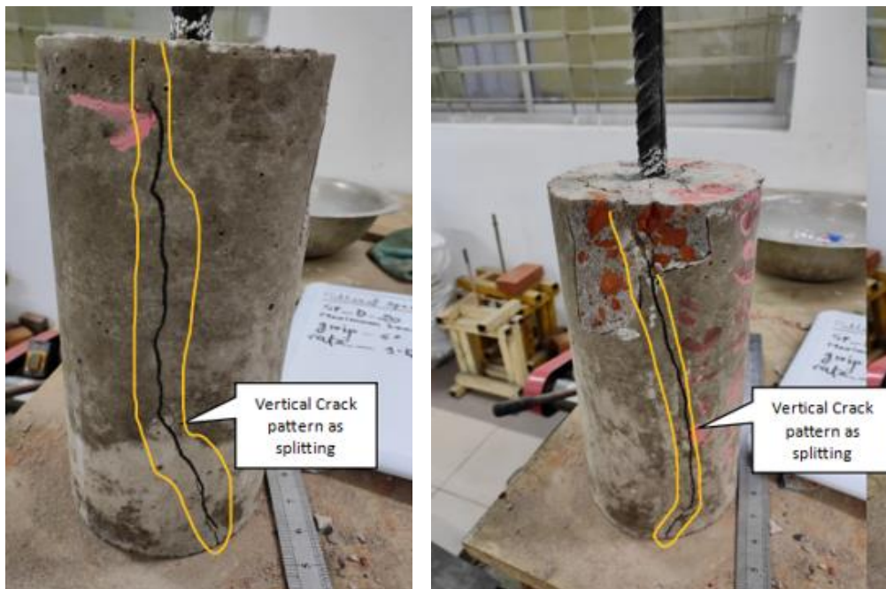
Fig. 9. Identification of Crack Pattern of Pullout Specimen, SP-D-20 (1.6'')
